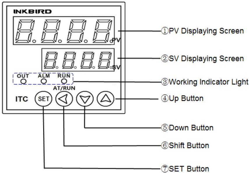
① **PV Displaying Screen:** Displaying the measuring value or the setting parameters.
